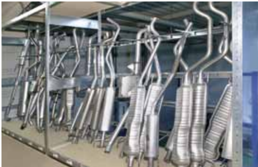
Exhaust pipes tidily arranged and separated by rod dividers
