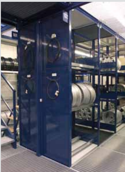
Wheels are held on special depth-adjustable supports
