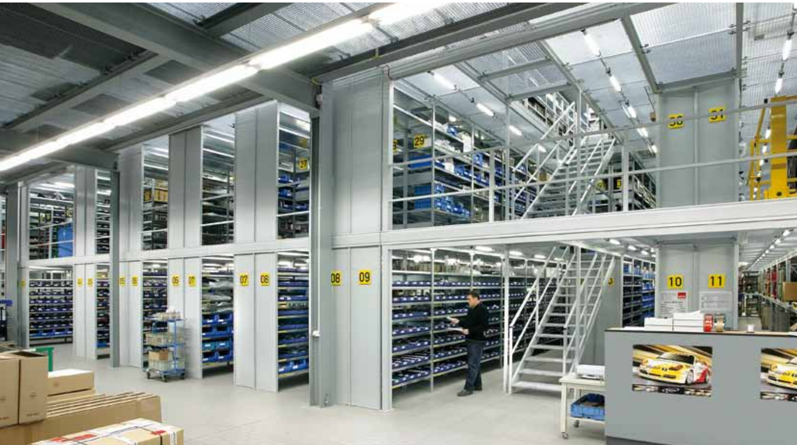
3-tier storage facility in the automotive industry
