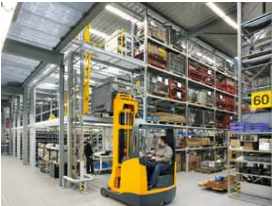
META QUICK® shelving system with META MULTIPAL® pallet racking system and integrated loading station
