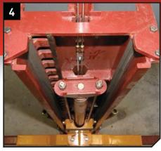
▲ Heavy duty column construction with direct drive cylinders, direct drive lifting rods (not cables) and stainless steel hydraulic lines (not rubber hoses) which will never wear.
