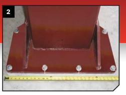
▲ Mohawk's large and stable footprint measures 30" wide by 24" is made of ¾" thick plate. Mohawk's large base gives stability to the lift, while distributing the load to the shop floor.
