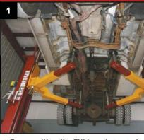
▲ Two post lifts offer **FULL unobstructed unvehicle access** for all repairs, take up minim space and leaves wheels hanging free for tiror any other necessary repairs.
